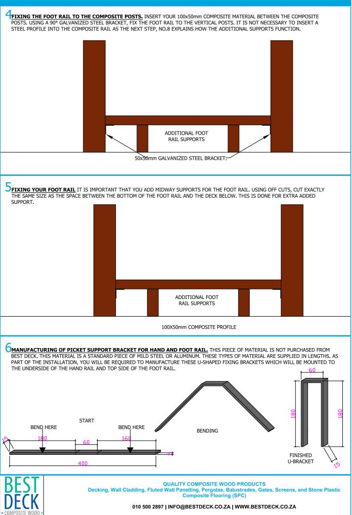
**FIXING THE U-SHAPED BRACKET TO THE FOOT RAIL** THIS BRACKET WOULD BE SCREWED DOWN TO THE COMPOSITE FOOT RAIL. ENSURE 2x FIXING SCREWS ARE USED THROUGH THE BASE OF THE BRACKET, ENSURING THAT THE BRACKET IS SECURELY FIXED AND DOESN'T PIVOT SO THAT ONCE THE COMPOSITE PICKET IS SLID OVER THE U-BRACKET, IT IS NICE AND TIGHT.
