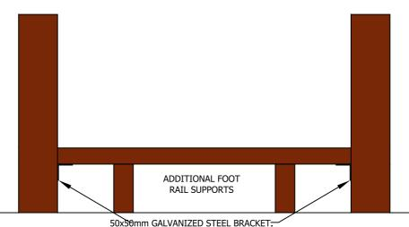
5 FIXING YOUR FOOT RAIL IT IS IMPORTANT THAT YOU ADD MIDWAY SUPPORTS FOR THE FOOT RAIL. USING OFF CUTS, CUT EXACTLY THE SAME SIZE AS THE SPACE BETWEEN THE BOTTOM OF THE FOOT RAIL AND THE DECK BELOW. THIS IS DONE FOR EXTRA ADDED
