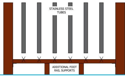
INSERTING YOUR HAND RAIL OVER THE STAINLESS STEEL TUBES. DRILLED TO THE UNDERSIDE OF YOUR HAND RAIL ARE THE HOLES FOR THE STAINLESS STEEL TUBES. WITH THE TUBES NOW IN PLACE, SIMPLY DROP THE HAND RAIL OVER THE TUBES THAT WILL SLOT INTO THE HOLES YOU HAVE DRILLED. AT THIS STAGE, ONE WOULD ALSO FIX THE 30x19 STEEL TUBE THAT RUNS THROUGH THE HAND RAIL TO THE VERTICAL POSTS AS PER DIAGRAM 8.
