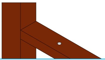
8 INSERTING THE HAND RAIL. INSERT A 30x19x1.2mm PRIMED (INSIDE AND OUTSIDE) STEEL TUBE DOWN THE CENTER CAVITY OF THE COMPOSITE PROFILE. NOTCHING OUT THE COMPOSITE POST AND STEEL TUBE INSERT TO LAY THE 30x19mm TUBE ON. THIS WHAT SUPPORTS YOUR HAND RAIL.
