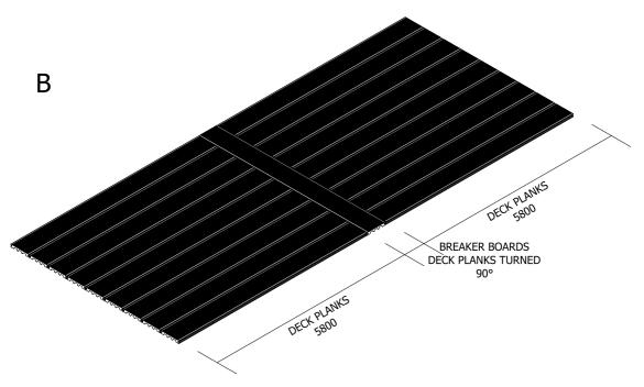
USING A BREAKER BOARD IS ESSENTIAL TO ENSURING AN AESTHETICALLY PLEASING COMPOSITE DECK.
