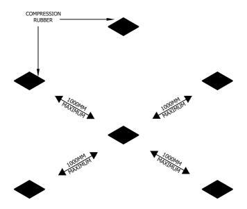
COMPRESSION RUBBER LAYOUT. LAY AND BOND YOUR 6mm COMPRESSION RUBBER USING A WATERPROOF ADHESIVE WHERE THE BASE PLATES WILL BE SITUATED. ENSURE COMPRESSION RUBBER EXCEEDS BASE PLATES SIZE BY AT LEAST 25mm ALL THE WAY AROUND. ONCE THE DECK STRUCTURE AND PLANKS HAVE BEEN FITTED, EVERYTHING WILL STAY IN PLACE UNDER ITS OWN WEIGHT.
