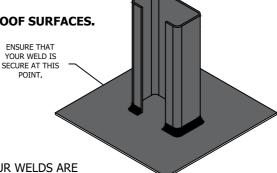
**WELDING C-CHANNEL TO BASE PLATE.** ENSURE THAT YOUR WELDS ARE SECURE AND A RUST PRIMER IS TO BE APPLIED TO ALL WELDS.
