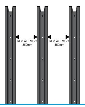
FIXING THE C-CHANNELS TO THE STRUCTURE. FASTEN THE 64x32x2mm TOP HAT PROFILE TO YOUR WALL USING FISCHER HAMMER FIXINGS. THE FISCHER FIXINGS SHOULD BE FASTENED AT EVERY 400mm THROUGH THE TOP HAT PROFILE, WITH THE TOP HAT PROFILE SPACED AT 350mm APART OR LESS. IT IS IMPORTANT TO ENSURE THAT ALL JOISTS ARE ALL PERFECTLY FLAT, STRAIGHT AND LEVEL.
