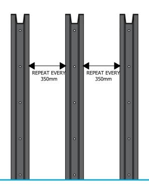
FIXING THE C-CHANNELS TO THE STRUCTURE. FASTEN THE 64x32x2mm TOP HAT PROFILE TO YOUR WALL USING FISCHER HAMMER FIXINGS. THE FISCHER FIXINGS SHOULD BE FASTENED AT EVERY 400mm THROUGH THE TOP HAT PROFILE, WITH THE TOP HAT PROFILE SPACED AT 350mm APART OR LESS. IT IS IMPORTANT TO ENSURE THAT ALL JOISTS ARE ALL PERFECTLY FLAT, STRAIGHT AND LEVEL.
